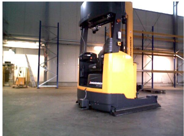
**Figure 1:** An automated reach truck in a warehouse serving as test environment.
