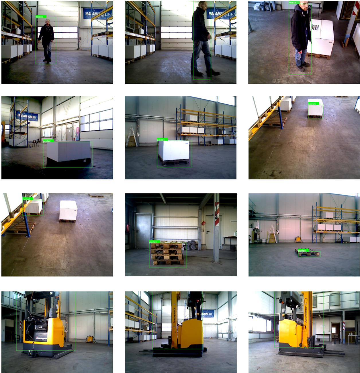
**Figure 4:** Results obtained on the validation dataset captured in a warehouse environment. Our system is able to detect and recognize objects of the classes: *forklifts*, *humans* and *palletted goods* under varying poses and illumination conditions.
