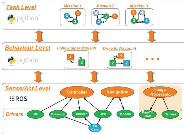
**Figure 6:** Software architecture of the MONSUN underwater robot subdivided into three levels.
