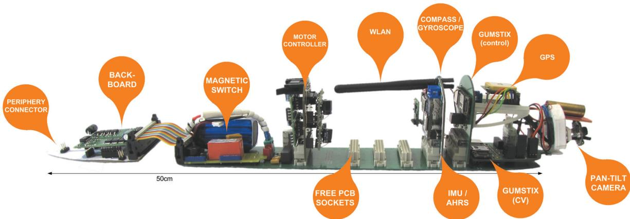
**Figure 4:** The MONSUN electronics designed as a bus-based architecture. Different pcb-boards equipped with controllers and sensors can be placed at various available sockets to achieve a high flexibility for different mission tasks. Due to the fact of uniform boards, they can be exchanged between different robots for a fast reaction to failure cases.
