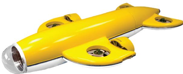
**Figure 1:** The MONSUN Underwater Robot designed for applications like environmental monitoring tasks in a swarm. It has a small size with a length of 60 cm and a diameter of 10 cm, which makes it easy to handle by one person.
