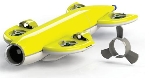
**Figure 3:** The CAD model of MONSUN including the new 3D printed propeller developed in *Solidworks*.
