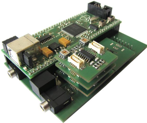
**Figure 5:** The acoustic modem for MONSUN assembled on an evaluation board. Modular PCB boards containing filter and amplification parts can be connected in a predefined way to perform first analogue preprocessing of the acoustic signals.
