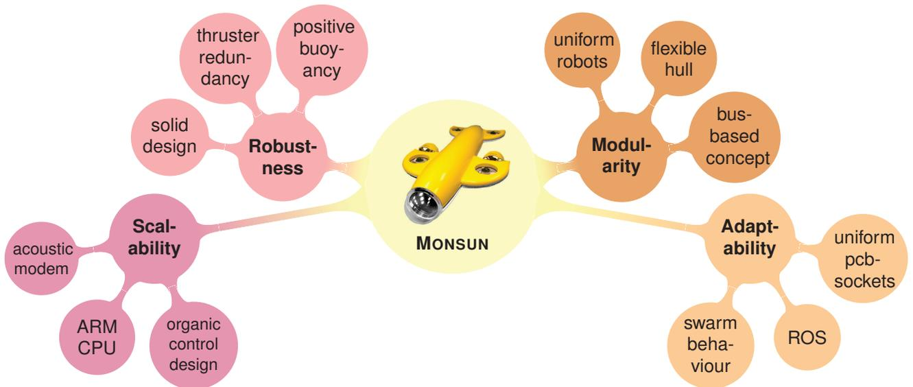
**Figure 2:** Conceptual design of the MONSUN autonomous underwater vehicle. It is characterized by a robust and modular design which makes it adaptive to many possible mission tasks. Due to the controllability in a swarm, the full design is scalable to a high number of swarm members achieved by high processing and communication capabilities.
