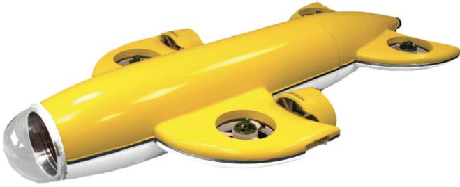
Fig. 3. The AUV MONSUN in its base version features small size and high agility. Four brushless motors in the fins for vertical and two motors for horizontal propulsion allow MONSUN to control its pose very accurately.
