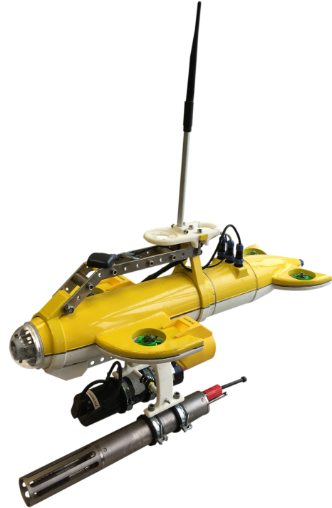
Fig. 1. The MONSUN underwater robot developed by the Institute of Computer Engineering of the University of Lübeck. With a length of 80 cm, it is small in size and actuated with six brushless motors, four directed in the vertical plane and two directed in the horizontal plane. They are placed at the fins enabling high maneuverability. For the behaviors described in this paper, it is equipped with a large antenna for WiFi communication at the surface and an acoustic modem at the bottom of the AUV at its right side (transducer not shown).
