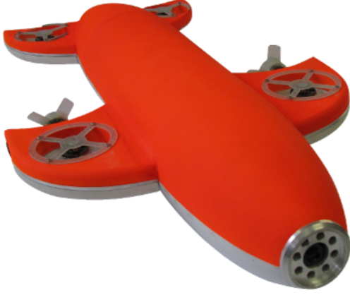
Fig. 1. The AUV MONSUN II with its small dimensions of a length of 60 cm and a diameter of 10 cm. The whole robot has a light weight of 4 kg and can be managed by a single person.
