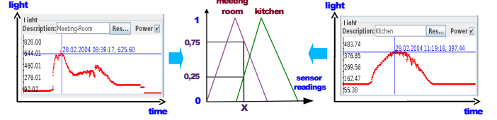
Fig. 2: Fuzzy-based sensor similarity computation.
